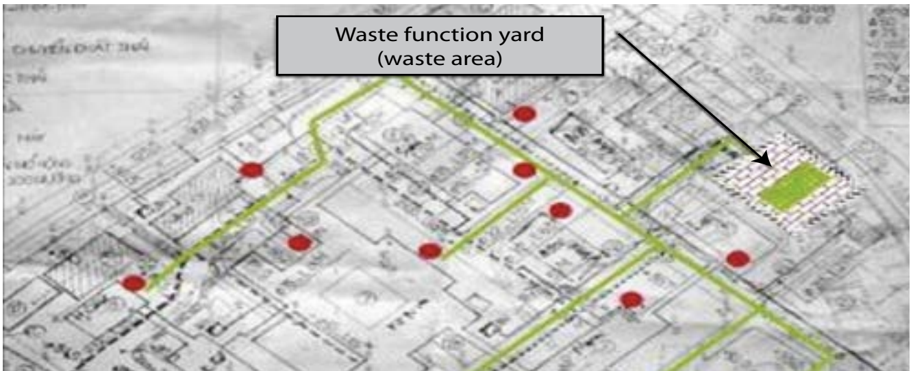
Figure 7.7 Example of a health-care facility site plan with waste-collection points (red circles)
