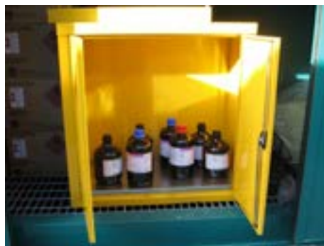
Inside a safety cabinet for flammable substances
